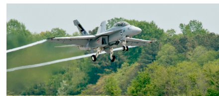
NAS Patuxent River and the Atlantic Test Ranges serve as an important flight testing site (top). Testing an F/A-18 Hornet that runs on 50% biofuel (bottom).
