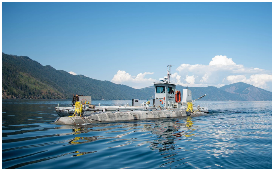
The Columbia-class submarine model Pike is towed through the waters of Lake Pend Oreille in Bayview, Idaho, by Naval Surface Warfare Center, Carderock Division personnel in August 2022. The command's Acoustic Research Detachment in Bayview is the Navy's hidden gem for acoustic testing because of its geographical location and quiet waters.
