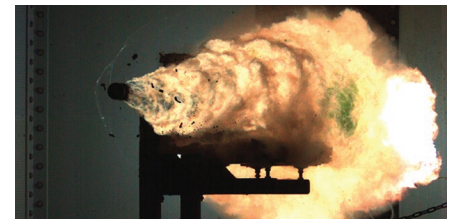
Research, development, test, and evaluation activities include the testing of unmanned aerial vehicles (top), as well as electromagnetic railgun, a long-range weapon that fires projectiles using electricity (bottom).
