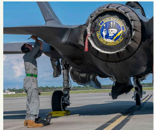
LO specialists conduct post-operations servicing outer mold line inspections on F-35A Lightning IIs after every flight to identify any possible damage in the aircraft coating. (U.S. Air Force photo by Tech. Sgt. Betty R. Chevalier)
